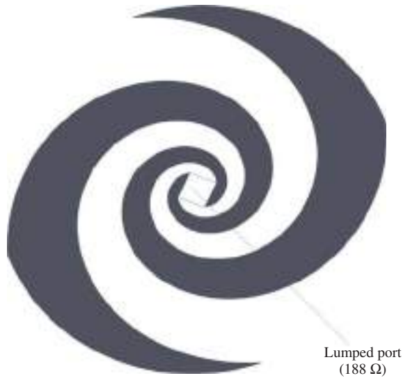
Figure 6.47 Simulation model of the logarithmic spiral antenna in Ansoft HFSS
