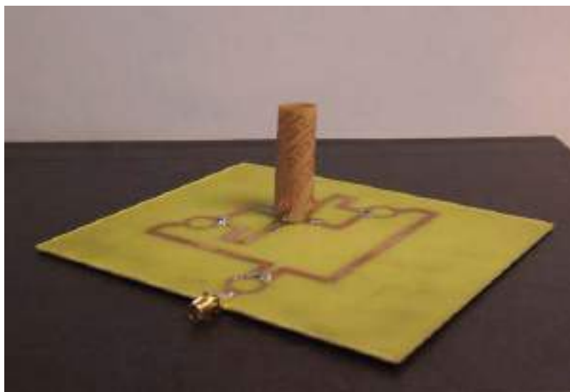
Figure 6.15 Photo of the fabricated MVPQHA with feed network [6] Reproduced with permission of © 2009 IEEE
