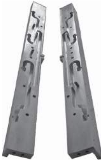
Figure 5.15 A photo of the fabricated feed network for the waveguide-fed CP microstrip array [12]. Reproduced with permission of © 2005 IEEE
