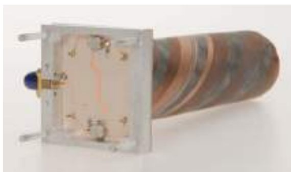
Figure 3.39 Prototype of a broadband folded PQHA with a wideband feeding circuit [45]. Reproduced with permission of © 2010 IEEE
