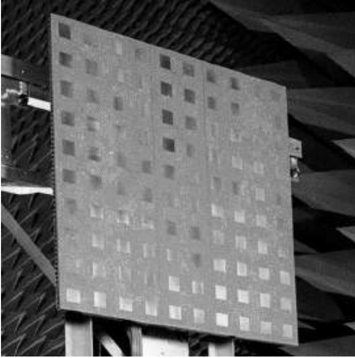
Figure 14.38 Antenna array of 10 \times 10 rectangular microstrip patches, 2–2.3 GHz, for space-to-space communications. (Courtesy: Ball Aerospace & Technologies Corp.)
